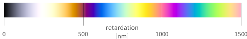
Bild 3 Interference colour chart according to Michel-Lévy (analytical calculation) [7]
