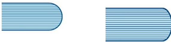
Figure 9 Pencil edge , LHS half-round, RHS flat round
