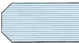
Figure 6 Smooth ground edge
